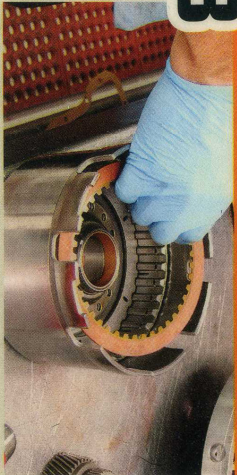
8 Brand-new clutches and steels are used throughout. Level 10 uses high-performance pieces and contributes the total torque capacity of a 4L60E/4L65E to the quality of the clutches and how well the valvebody and front pump are modified. Because our reverse-input drum was badly worn, we had to replace it with a new one. No worries for us, as Level 10 is used to this kind of carnage and promptly pulled one off its shelves and put it on our tab.
