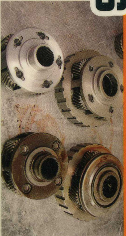
6 Using four-pinion planetary gearsets, 4L60E transmissions can handle a good amount of power and torque. But with the increased torque from our planned engine mods and the Caprice's portly weight, Pat recommended a 4L65E gearset, which incorporates five pinions in each assembly. This offers as much as a 25 percent greater torque capacity.
