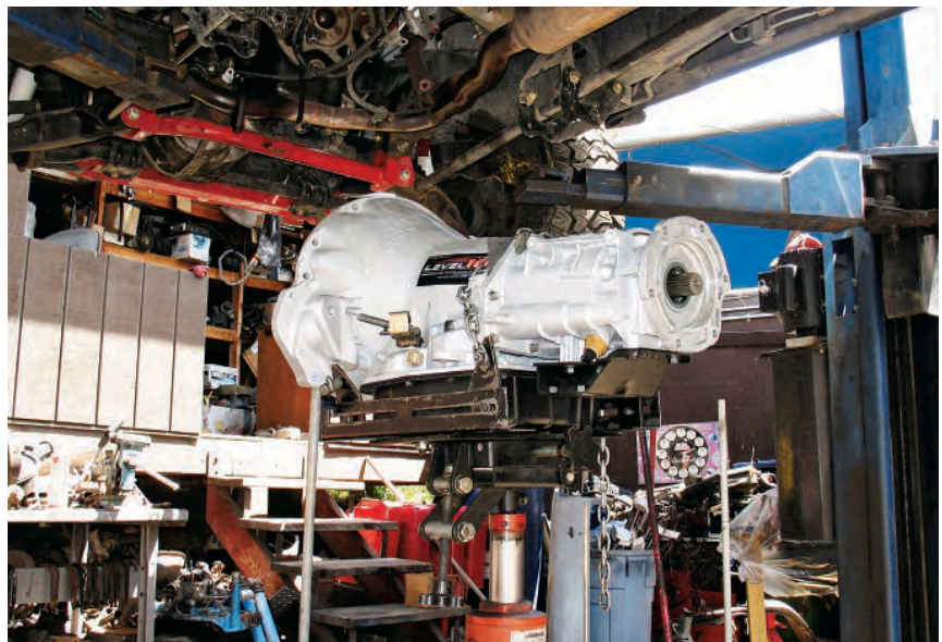
▲ With the transmission back in our hands, Abel Estrada of Jeeps R Us lifted the transmission onto the tranny jack and pumped the tranny up into place.
