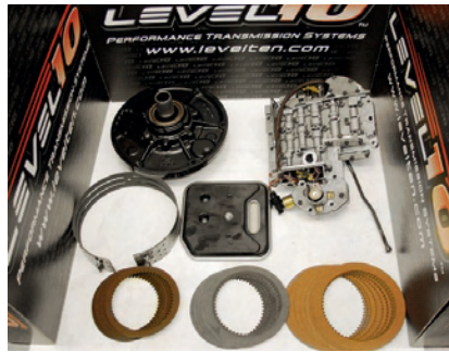
▲ Level 10's Master Kit for transmissions is dubbed 'The Animal' build kit. It includes the Superpump, high-energy clutches and bands, new seals, gaskets, and the modified valvebody.
